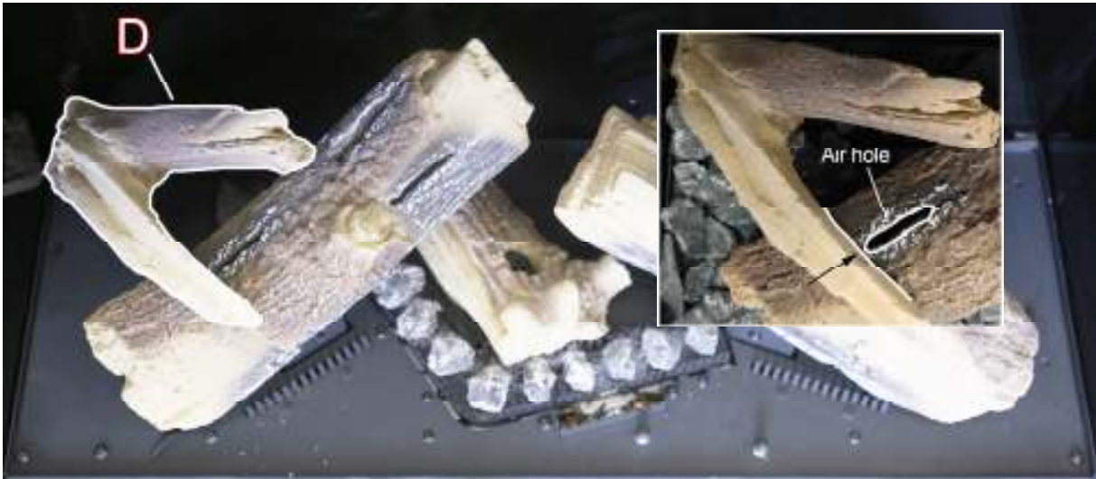
Place Log D in the orientation shown ensuring the branch sits just in front of the air hole
